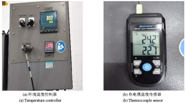
图 5 环境温度控制器及热电偶传感器 Fig.5 Environmental temperature controller and thermocouple sensor
