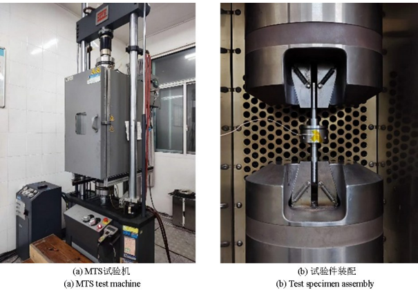
图 4 耗散特性试验设备及装配 Fig.4 Dissipation characteristic test equipment and assembly
