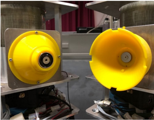
图 12 电磁对接机构 3D 打印实物 Fig.12 Electromagnetic docking mechanism by 3D printing
