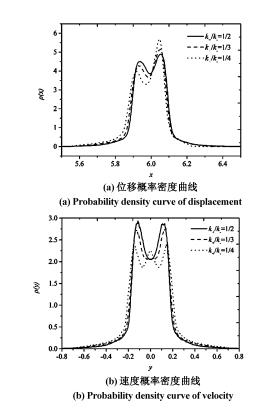
图 7 拉压刚度比  $k_+/k_-$  取不同值时的稳态响应概率密度不同 Fig. 7 Probability density of stationary response for different values of stiffness ratio  $k_+/k_-$
