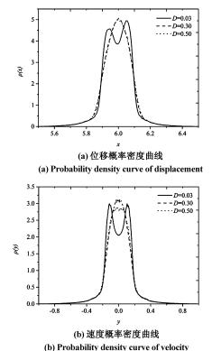
图 8 激励强度 D 取不同值时的稳态响应概率密度 Fig. 8 Probability density of stationary response for different values of excitation intensity D
